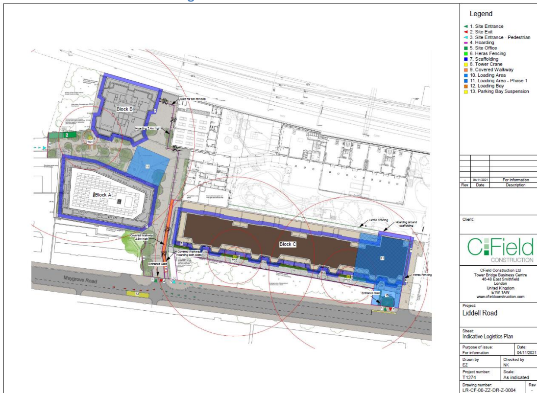
Figure 7 – Construction Site Plan
