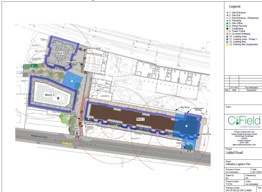
Figure 7 – Construction Site Plan
